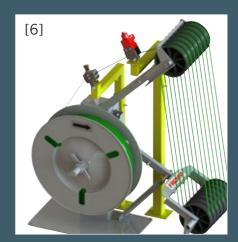
[6] End of Film or Strap signalling – visual, acoustic or electronic warning Informs the system or the operator direct, to reduce change time of strap or film.
