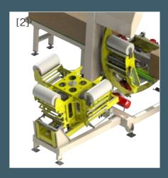
[2] Automatic Film roll change unit – for automatic wrapping machines
